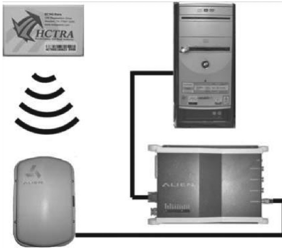
Figure 3.4 RFID system components. (From Erick C. Jones and Christopher A. Chung, RFID in Logistics: A Practical Introduction , Boca Raton, FL: CRC Press, 2008.)
